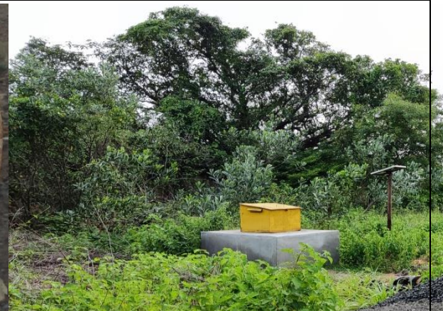
Piezometer for Ground water level (Online Station)
